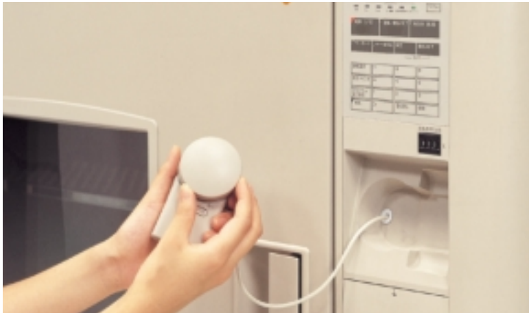
Jog dial for fine depressurization control
